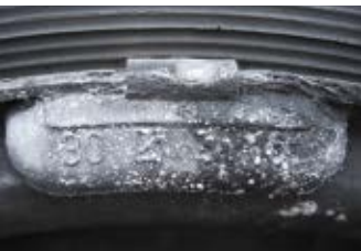
UNCOATED WEIGHTS: Contact corrosion of surface.
