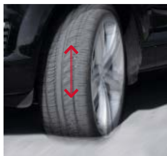
STATIC IMBALANCE: The wheel has a tendency to jump.
