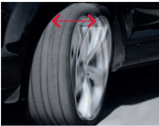
DYNAMIC IMBALANCE: The wheel has a tendency to wobble.
