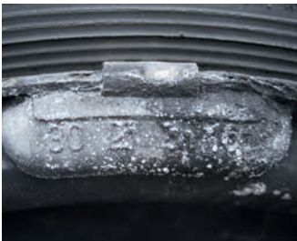
UNCOATED WEIGHTS: Contact corrosion of surface
