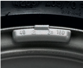
COATED WEIGHTS: Sealed epoxy finish. The result: no oxidation of surface.
