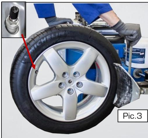
It is important that the TPMS Sensor is on the opposite side of the bead breaker, when the tyre is pressed down on the rim (see Pic.3).
